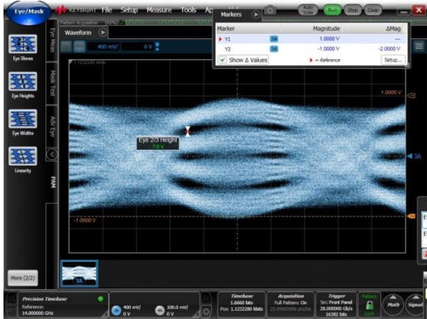
28 Gbaud With Emphasis (before passing -10 dB channel)
