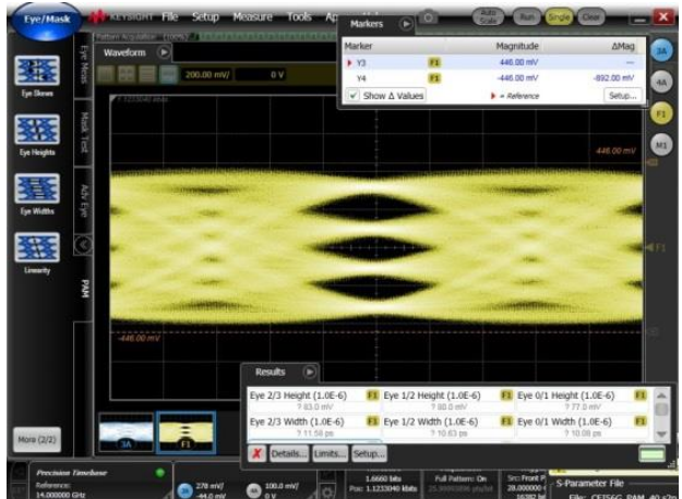
28 Gbaud With Emphasis (after passing -10 dB channel)
